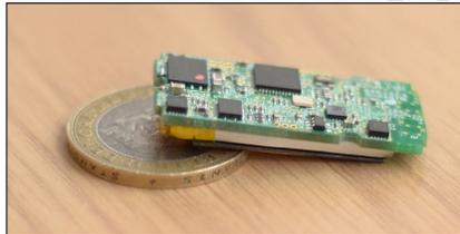
Figure 4: SPW-2: ARM Cortex-M3 based wearable accelerometer platform [32].
