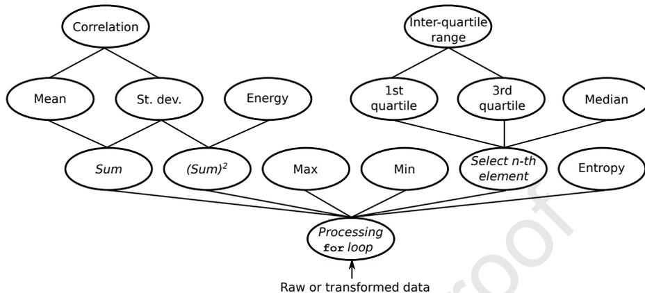
Figure 2: Features under consideration and their inter-dependencies. Labeled in *italics*: intermediate results that are included in the energy model, but not in the feature group selection stage.
